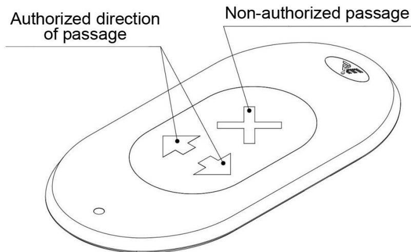
*Fig. 2 General view of LED panel*
