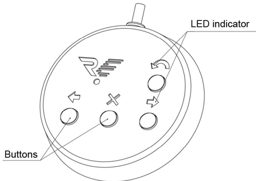
*Fig. 4 General view of remote control panel*
